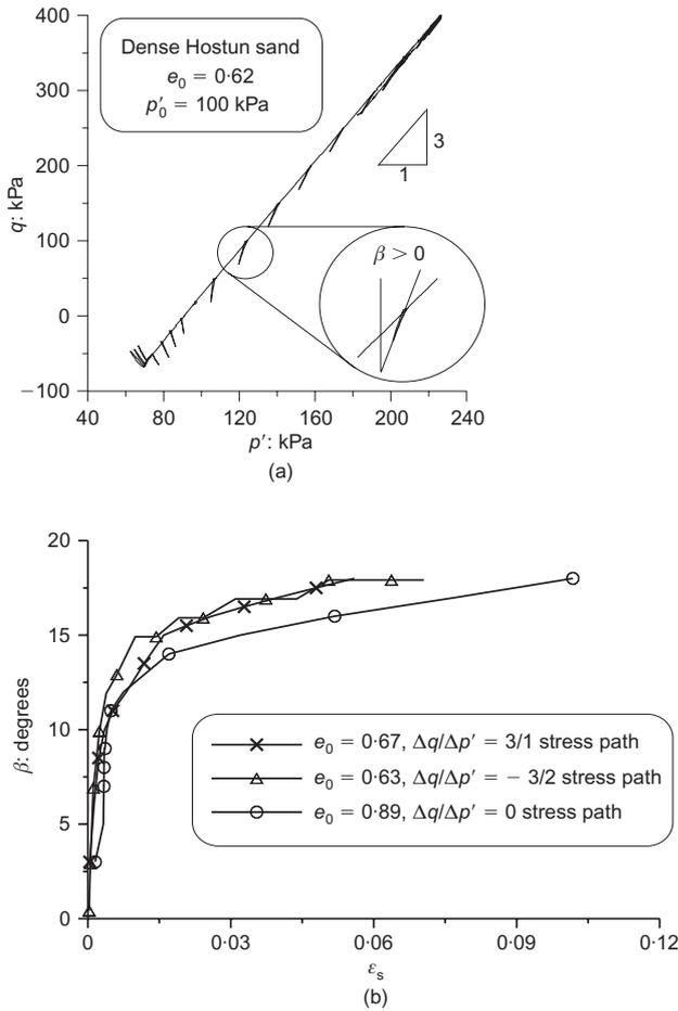
**Fig. 2. Experimental exploration of evolution of tangent elastic anisotropy in triaxial tests: (a) conventional drained test with initial extension stress state and definition of inclination  $\beta$  of effective stress path resulting from a small undrained unload-reload cycle; (b) evolution of tangent elastic anisotropy  $\beta$  with deviatoric strain for loose and dense sand along different compression loading paths**
