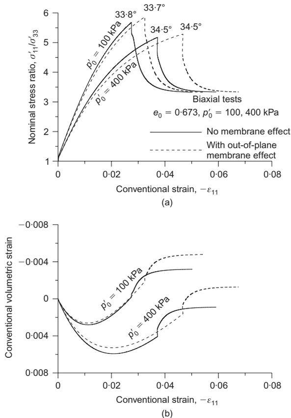
Fig. 14. Biaxial compression of dense sand, effects of out-of-plane stiffness on: (a) nominal stress ratio against conventional axial strain; (b) conventional volumetric strain against axial strain
