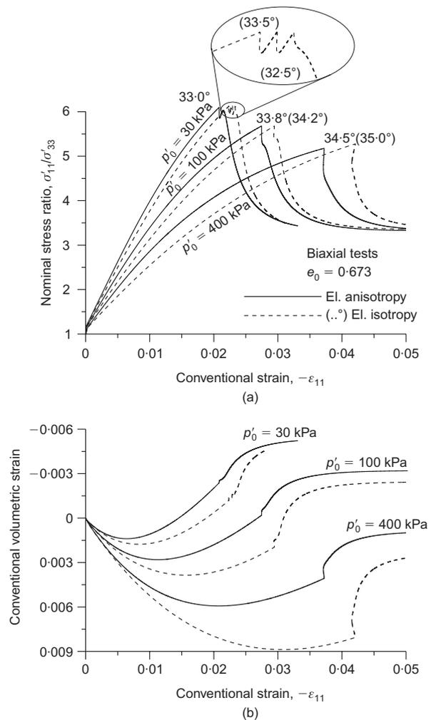
Fig. 10. Effects of elastic anisotropy on occurrence of strain localisation in drained biaxial compression tests performed at various confining pressures on dense sand: (a) nominal stress ratio against conventional axial strain; (b) conventional volumetric strain against axial strain
