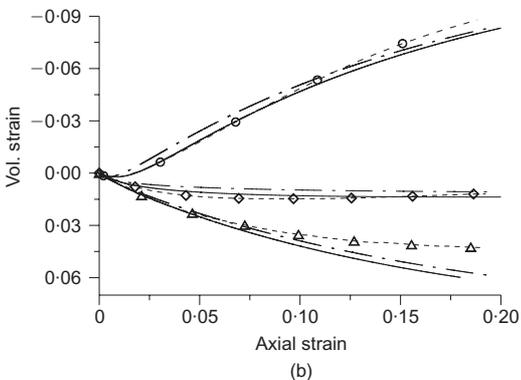
Fig. 5. Drained, conventional triaxial compression tests on Hostun sand RF (initial pressure  $p'_0 = 300$  kPa): experiments and simulations. Effect of choice of constitutive parameters: (a) deviatoric stress and axial strain; (b) volumetric and axial strain
