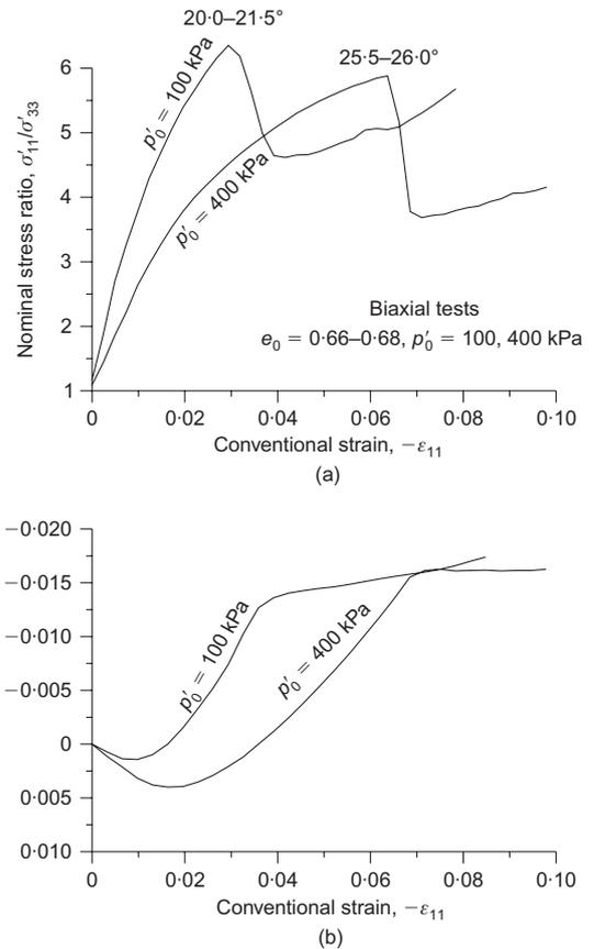
Fig. 15. Experimental results on samples of dense Hostun sand at different confining pressure: (a) nominal axial stress against conventional strain; (b) conventional volumetric strain against axial strain (from Desrues & Hammad, 1989)
