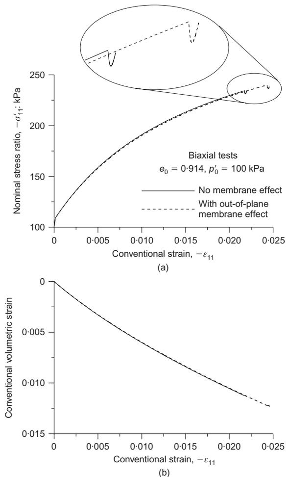
Fig. 16. Biaxial compression of loose sand, effects of out-of-plane compliance on: (a) nominal stress against conventional axial strain; (b) conventional volumetric strain against axial strain
