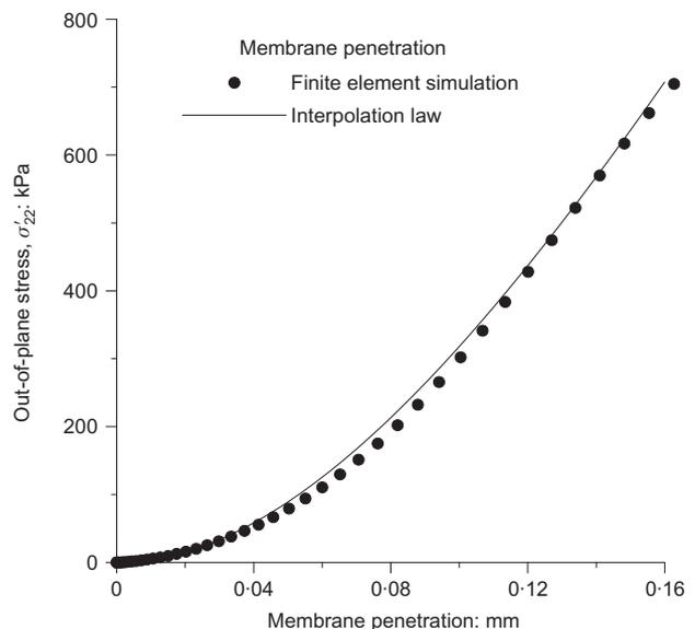
Fig. 13. Out-of-plane stress as a function of membrane penetration evaluated through finite-element modelling (Fig. 12)
