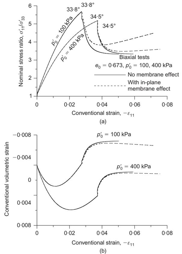
Fig. 17. Increase of apparent stiffness post-localisation due to membrane stretching. Biaxial compression of dense sand: (a) nominal stress ratio against conventional axial strain; (b) conventional volumetric strain against axial strain
