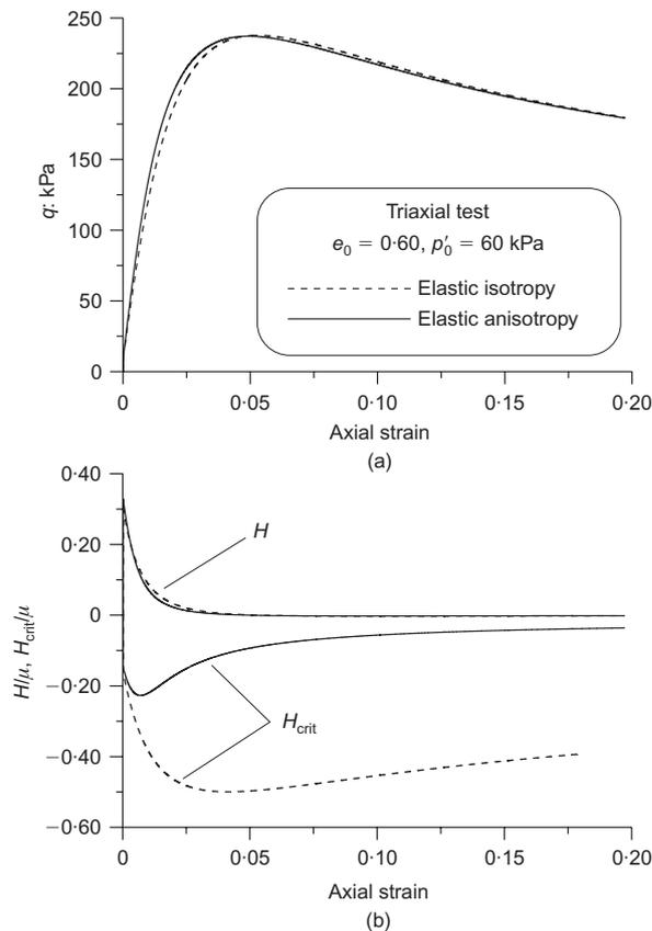
Fig. 9. Effects of elastic anisotropy on occurrence of strain localisation in a drained triaxial compression test on dense sand: (a) stress–strain behaviour; (b) evolution of hardening modulus for material, and critical hardening modulus for localisation
