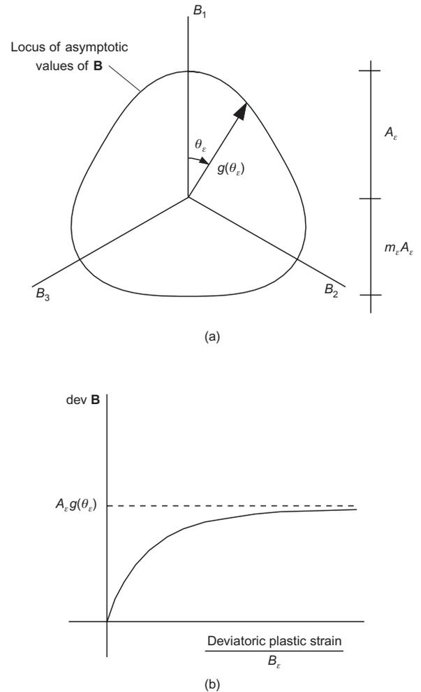
**Fig. 3. Elements of evolution of fabric tensor  $B$  defining elastic anisotropy and definition of corresponding constitutive parameters: (a) locus of asymptotic values of  $B$  in deviatoric plane; (b) monotonic variation of deviatoric component of  $B$  with deviatoric plastic strain with controlling parameter  $B_\epsilon$  and asymptote  $A_\epsilon$**
