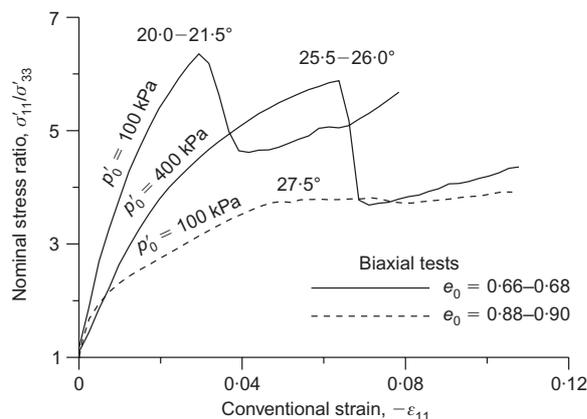
Fig. 7. Experimental results for compression of 350 mm high biaxial samples of dense and loose sand at different confining pressures (results taken from Desrues & Hammad, 1989)
