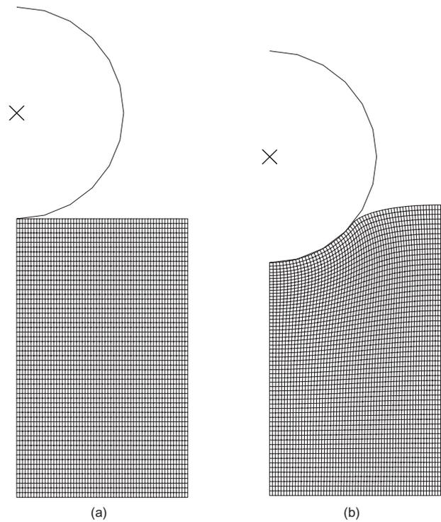
Fig. 12. (a) Undeformed and (b) deformed finite element mesh employed for evaluating penetration of rigid sphere of diameter 0.38 mm into 0.50 mm thick, neo-Hookean, incompressible, elastic support, with smooth constraint on lateral and bottom surfaces
