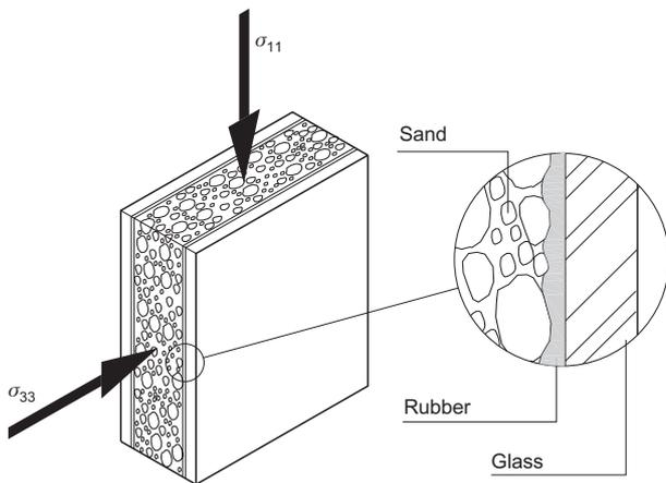
Fig. 11. Experimental arrangement for plane-strain tests
