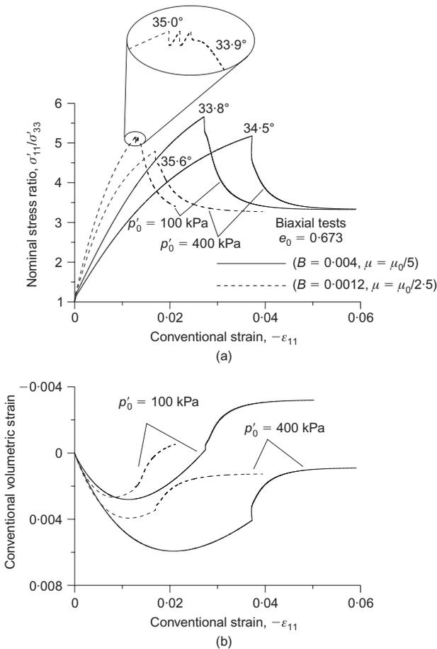
Fig. 8. Effects of choice of constitutive parameters on occurrence of strain localisation in drained biaxial compression tests performed at various confining pressures on dense sand: (a) nominal stress ratio against conventional axial strain; (b) conventional volumetric strain against axial strain
