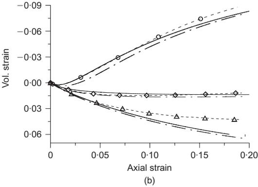
Fig. 4. Drained, conventional triaxial compression tests on Hostun sand RF (initial pressure  $p'_0 = 300$  kPa): experiments and simulations. Comparison of isotropic and anisotropic elasticity: (a) deviatoric stress and axial strain; (b) volumetric and axial strain
