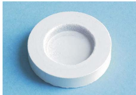
Fig. 17. Photograph of the formed green piece (5 g of M KMS-96 alumina powder has been used and a final mean pressure of 100 MPa has been reached).
