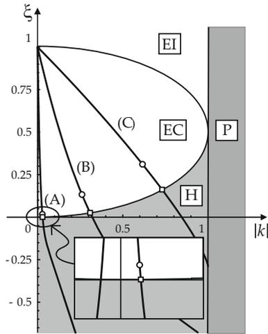
**Fig. 4** Deformation paths in the  $\xi-k$  plane for the GBG materials with the parameter combinations (A), (B) and (C) reported in Table 1. Note that  $\xi$  becomes negative at sufficiently high prestress  $k$
