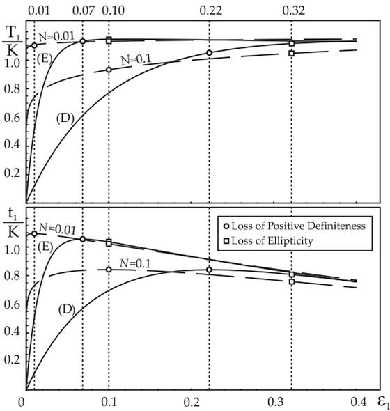
**Fig. 3** Uniaxial plane strain tension response for GBG material [selected with constants defined in Table 1 as (D) and (E)] and J<sub>2</sub>-deformation theory material (with  $N = 0.01$  and  $0.1$ ). Logarithmic strain  $\epsilon_1$  versus Cauchy stress  $T_1$  (upper part) and nominal stress  $t_1$  (lower part), normalized through division by  $K = 2,000$  MPa. Loss of positive definiteness of the elastic tensor and loss of ellipticity are marked with spots
