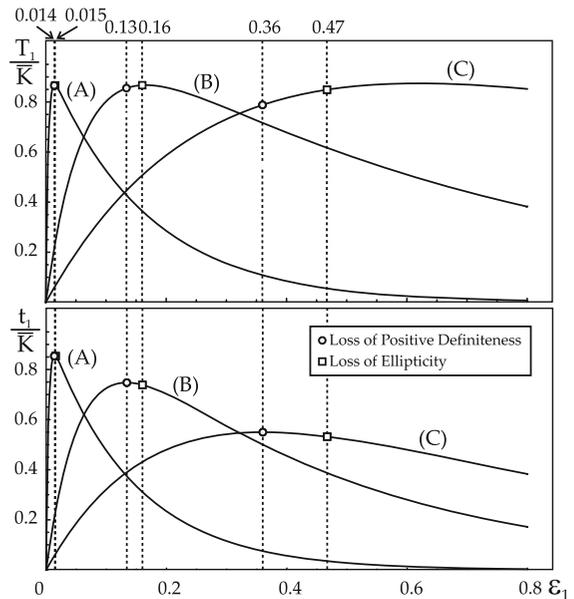
**Fig. 2** Uniaxial plane strain tension response for GBG material [selected with constants defined in Table 1 as (A), (B) and (C)]. Logarithmic strain  $\epsilon_1$  versus Cauchy stress  $T_1$  (upper part) and nominal stress  $t_1$  (lower part), normalized through division by  $\bar{K} = 2,000$  MPa. Loss of positive definiteness of the fourth-order incremental constitutive tensor [see Eqs. (21) and (22)] and loss of ellipticity are marked with spots
