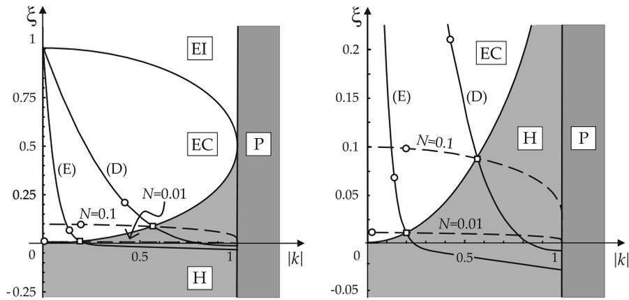
**Fig. 5** Stress paths in the  $\xi$ - $k$  plane for GBG material [with the parameter combinations (D) and (E) reported in Table 1] and  $J_2$ -deformation theory of plasticity ( $N = 0.1$  and  $N = 0.01$ ). Note that the anisotropization rate is higher in the latter material
