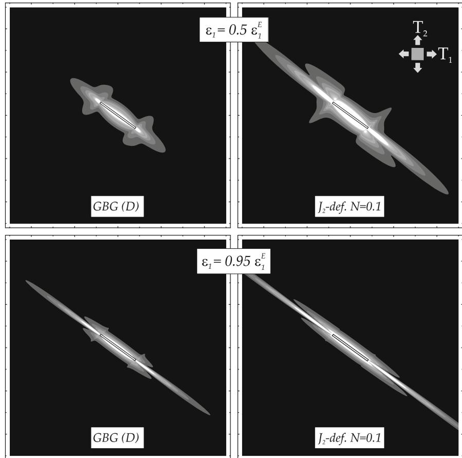
is a privileged mode of failure. On the other hand, the stiffer, Fig. 7, represents an obstacle to shear band propagation, so that the incremental deformation fields show that the band inclined with respect to the stiffener is almost completely inhibited, while that aligned ‘nearly parallel’ develops less than in the case of the slip surface.
