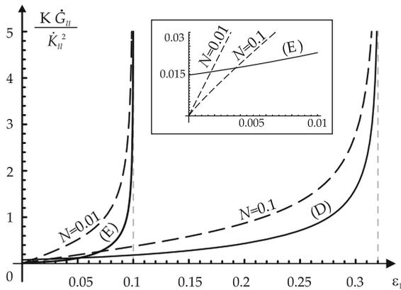
**Fig. 8** Mode II incremental energy release rate for slip surface growth in prestrained  $J_2$  [ $N = 0.01$  and  $N = 0.1$ ] and GBG [cases (E) and (D), Table 1] materials (prestrain parameter is  $\epsilon_1$ ). The slip surface is aligned parallel with a shear band direction. Note the difference between the two models in the rate of blow up, when the ellipticity limit ( $\epsilon_1 = \{0.1; 0.322\}$ ) is approached. A detail of the behaviour near the origin is shown in the inset
