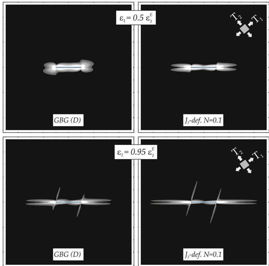
for an advance of the rigid line inclusion under Mode I, where
