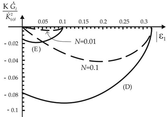
**Fig. 9** Mode I incremental energy release rate for rigid line inclusion reduction (negative growth) in prestrained  $J_2$  [ $N = 0.01$  and  $N = 0.1$ ] and GBG [cases (E) and (D), Table 1] materials (prestrain parameter is  $\epsilon_1$ ). The rigid line inclusion is aligned parallel with a shear band direction. Note the difference between the two models in the rate of decay to zero, when the ellipticity limit ( $\epsilon_1 = \{0.1; 0.322\}$ ) is approached
