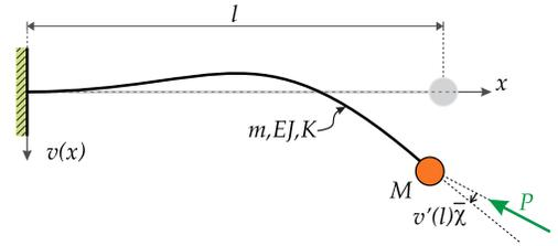
FIG. 1. The Pflüger column [53] clamped at  $x = 0$  with a point mass  $M$  at  $x = l$ . The column is loaded at  $x = l$  with a constant compressing circulatory force  $P$  inclined to the tangent to the elastic line of the column, so that  $v'(l)\chi = \text{const.}$  (equal to 0.092 in all the experiments).
