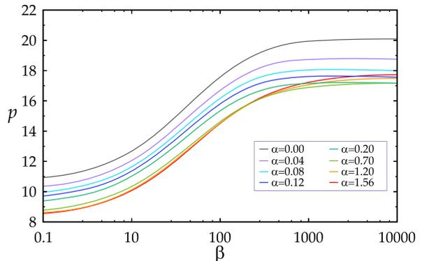
FIG. 5. Each curve, computed with the use of the equation (23), shows the critical flutter load in the limit of vanishing dissipation as a function of the damping ratio  $\beta$  for the discretized model with  $N = 2$  and  $\chi = 1$  and corresponds to a different mass ratio  $\alpha$  (reported in the legend). Note that at large mass ratios  $0.7 \lesssim \alpha \leq \pi/2$  the curves form a dense family.
