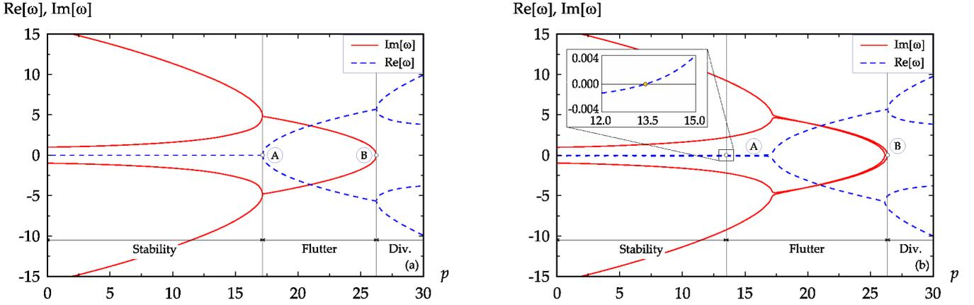
FIG. 7. Pulsation (red solid curves) and growth rates (blue dashed curves) for the Pflüger column versus the dimensionless load  $p$  (a) without damping and (b) in the presence of a Kelvin-Voigt damping for the material ( $\eta$ ) and air drag ( $\gamma$ ), demonstrating the drop in the onset of flutter. The plots were obtained with the parameters representative of sample 5 in Table I.
