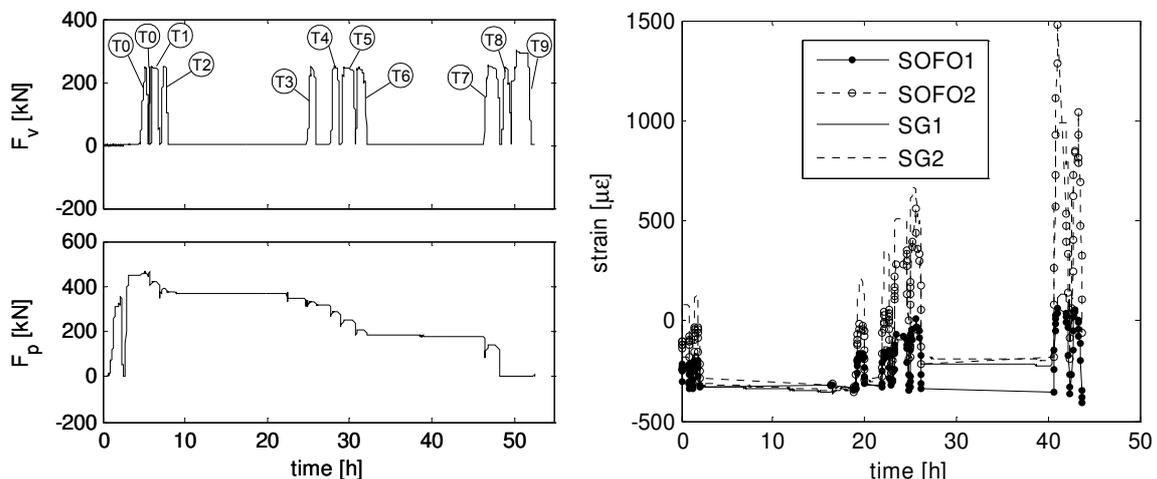
Fig. 2 (a) Load history applied to the element; (b) Time history recorded by SOFO system and strain gauges (SG).
