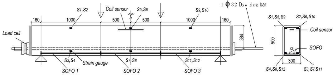
Fig. 1 Side view and cross section of the prototype of smart element.
