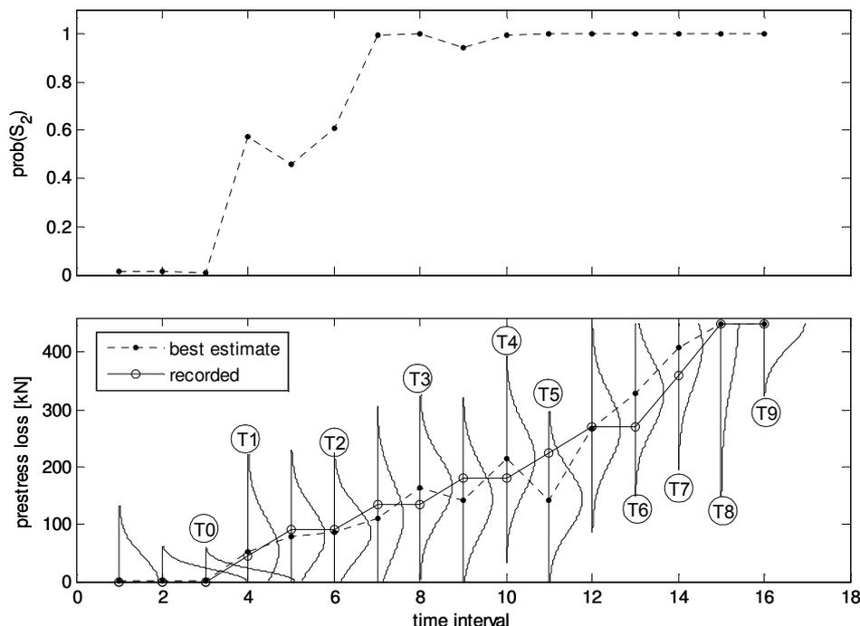
Fig. 4 Probability of scenario  $S_2$  at different time intervals (top); comparison between the estimated prestress loss and that recorded at the load cell (bottom).
