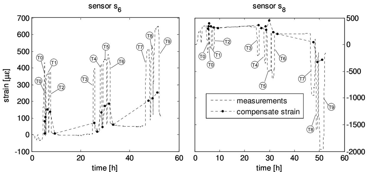
Fig.3 Estimated compensated strains for sensors 6 and 8.
