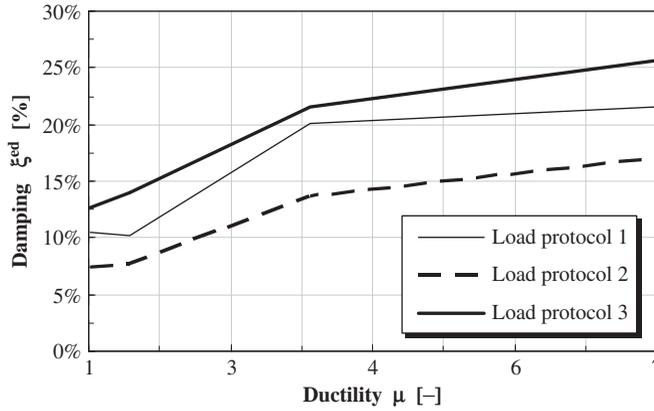
**FIGURE 8** Experimental equivalent damping vs. ductility relationships for ductile joints with 12 mm diameter dowels, based on Sartori [2008].
