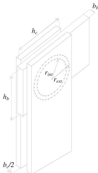
**FIGURE 4** Moment resisting joint.
