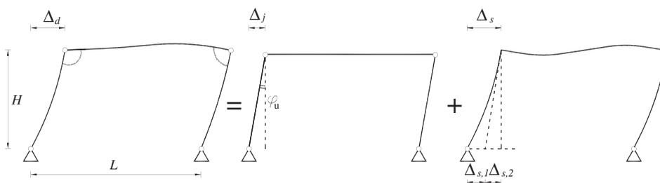
FIGURE 5 Conceptual model for estimating the target displacement.
