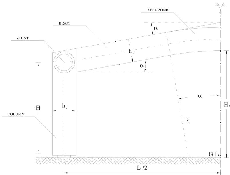
**FIGURE 2** Geometric features of the prototype portal.
