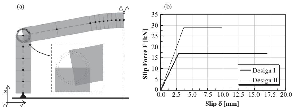
**FIGURE 10** Finite element model for nonlinear time pushover analysis (a) and load–slip model for  $d = 12$  mm (*Design I*) and  $d = 16$  mm (*Design II*) dowels (b).
