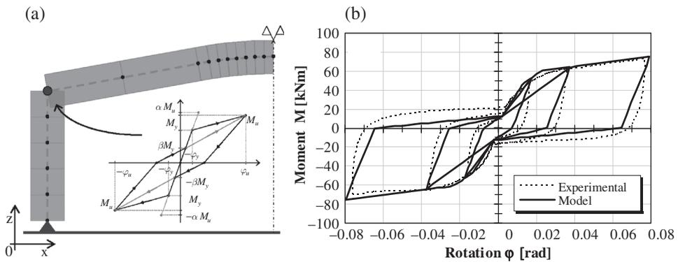
FIGURE 12 Finite element model for nonlinear time-history analysis (a) and moment-rotation relationship for the nonlinear rotational spring (b) compared with the experimental dataset from Polastri *et al.* [2008].
