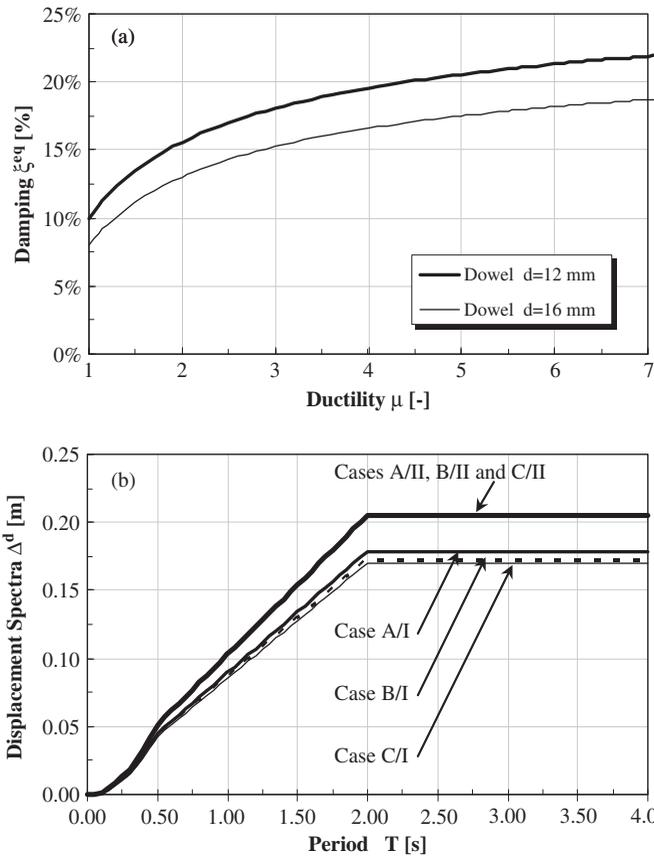
**FIGURE 9** Equivalent damping vs. ductility relationship (a) – Design displacement spectra (b).
