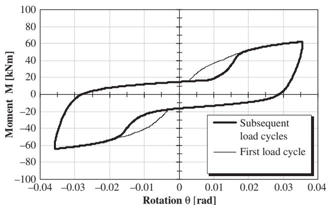
**FIGURE 7** Typical moment-rotation relationship for a doweled joint at first and subsequent load cycles, based on Polastri *et al.* [2008].
