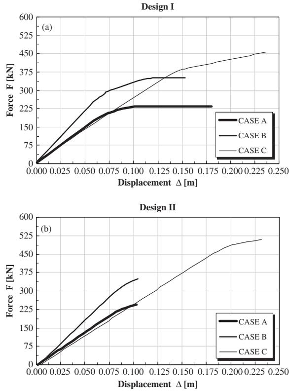
FIGURE 11 Pushover analysis of the portal under *Design I* (a) and *Design II* (b) assumptions.
