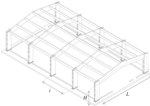
**FIGURE 1** Structure of portal timber frame building selected as case study [Piazza *et al.*, 2005].
