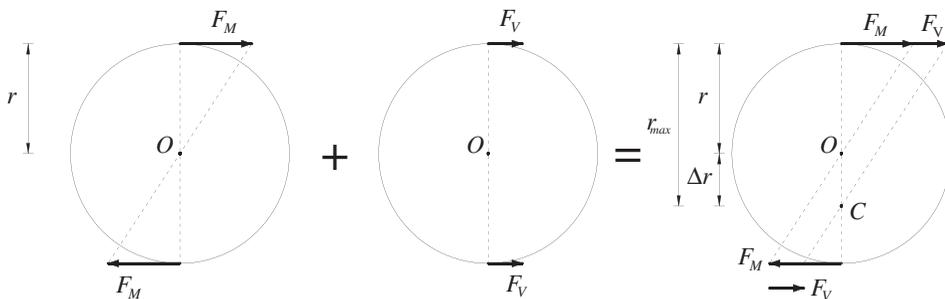
**FIGURE 6** Moment and shear stress components on dowels.
