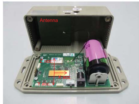
Fig. 3. Packaged accelerometer module with indication of axes.
