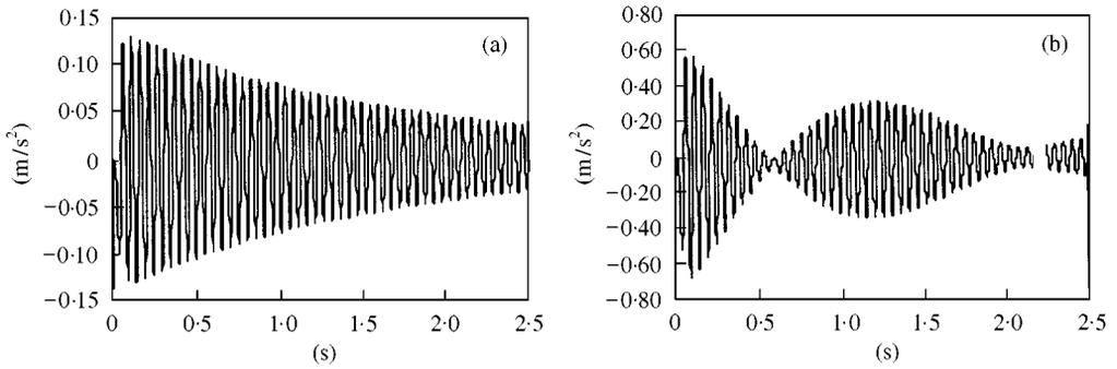
Figure 1. Free response of a PRC specimen: (a) undamaged; (b) cracked.
