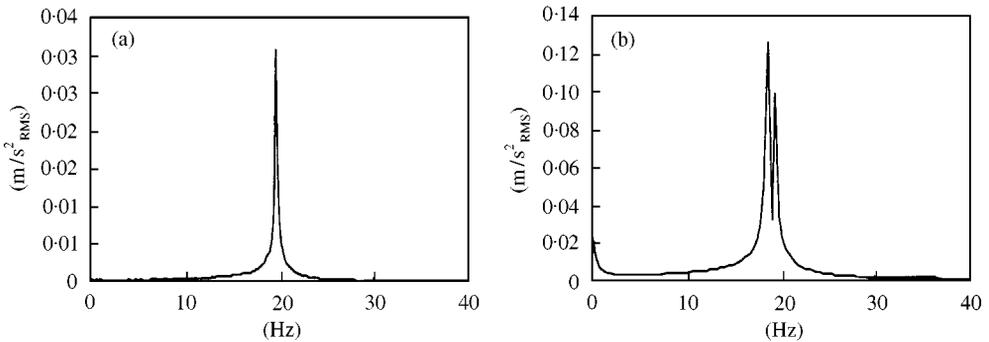
Figure 2. Free response FFT of a PRC specimen: (a) undamaged; (b) cracked.
