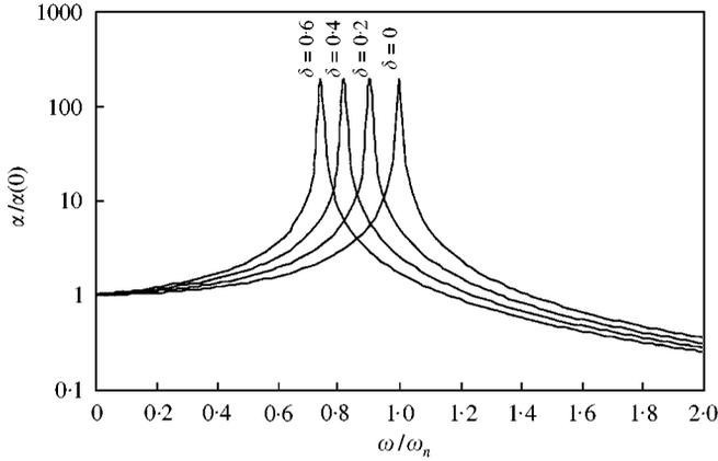
Figure 5. FRF of a dispersive oscillator for different values of the dispersion rate.
