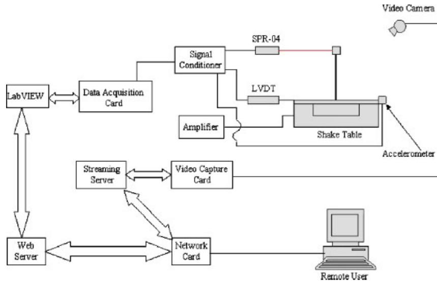
**Figure 4** Schematic of the Webshaker site. [Color figure can be viewed in the online issue, which is available at [www.interscience.wiley.com](http://www.interscience.wiley.com).]
