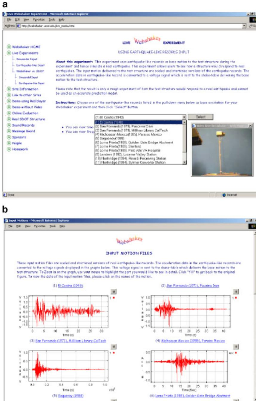
**Figure 5** (a) Earthquake-like base excitation. (b) Time history plots of four of the available earthquake-like motions. [Color figure can be viewed in the online issue, which is available at [www.interscience.wiley.com](http://www.interscience.wiley.com).]
