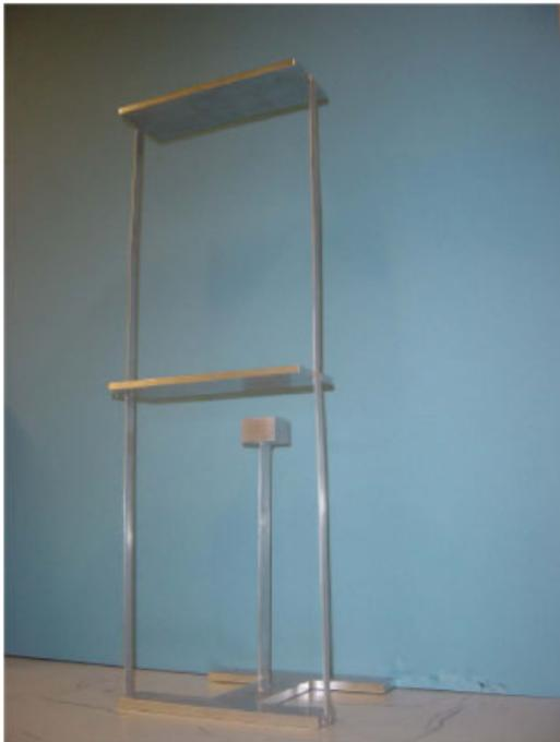
**Figure 8** (a) Aluminum single-degree-of-freedom inverted pendulum model. (b) Two-story aluminum frame model. [Color figure can be viewed in the online issue, which is available at [www.interscience.wiley.com](http://www.interscience.wiley.com).]
