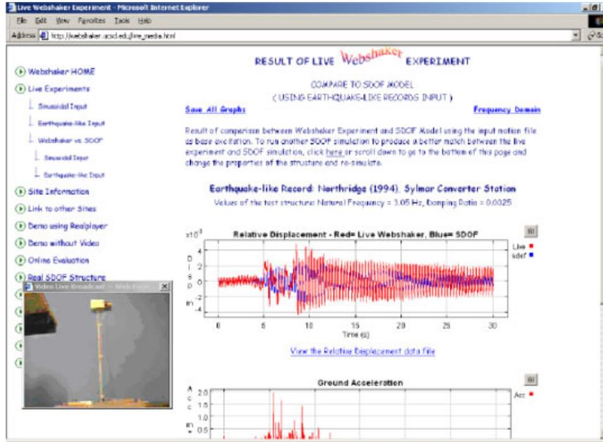
**Figure 7** Comparison between recorded data and numerical modeling. [Color figure can be viewed in the online issue, which is available at [www.interscience.wiley.com](http://www.interscience.wiley.com).]
