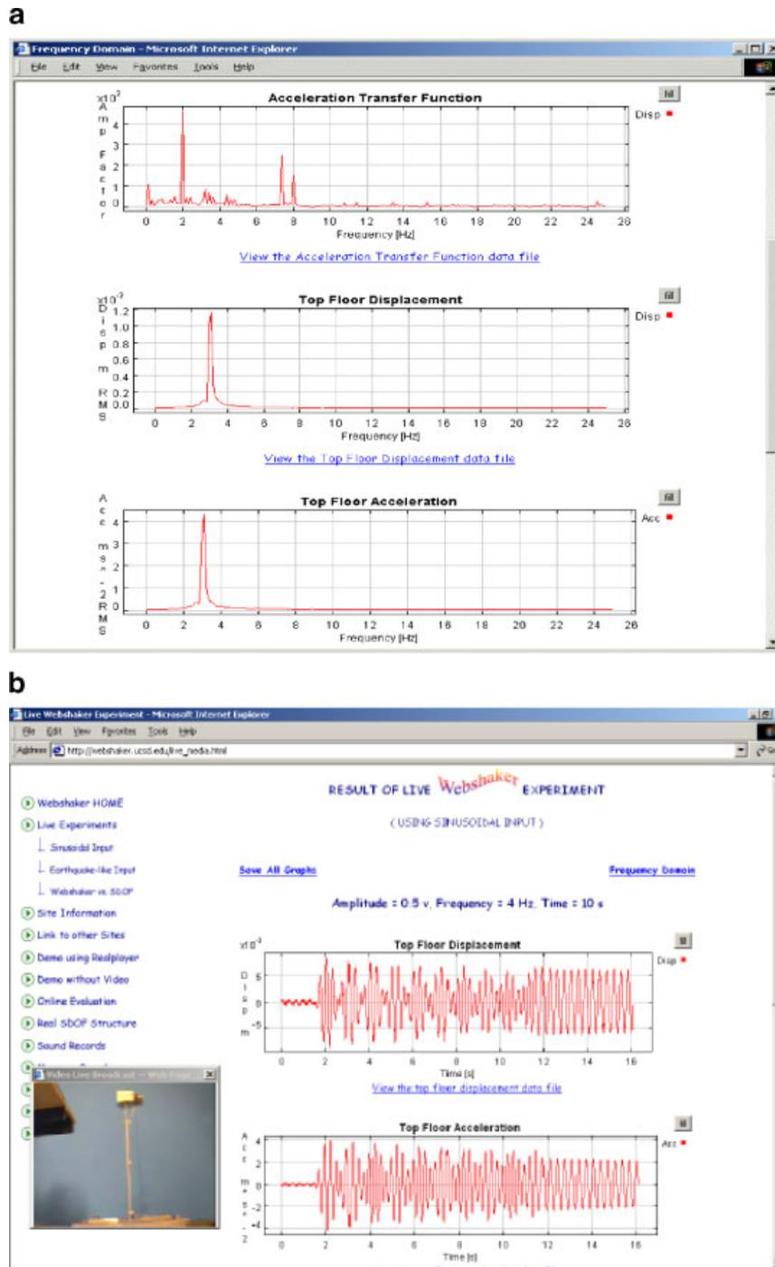
**Figure 6** (a) Frequency-domain form of recorded data and acceleration transfer function. (b) Graphical representation of recorded data. [Color figure can be viewed in the online issue, which is available at [www.interscience.wiley.com](http://www.interscience.wiley.com).]
