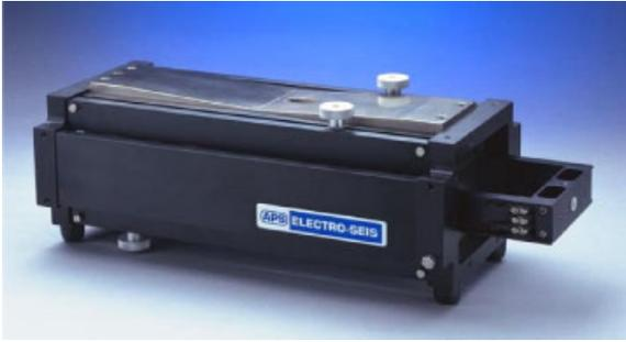
**Figure 2** APS Model 113-HF shake-table. [Color figure can be viewed in the online issue, which is available at [www.interscience.wiley.com](http://www.interscience.wiley.com).]
