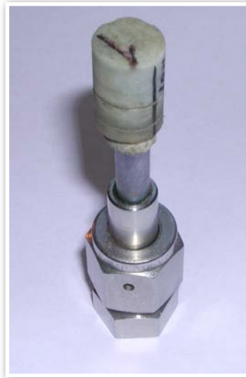
Figure 4: The quartz textured sample mounted for the experiment.
