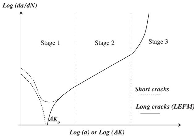
Fig. 3. A schematic of the typical fatigue growth behavior of cracks.
