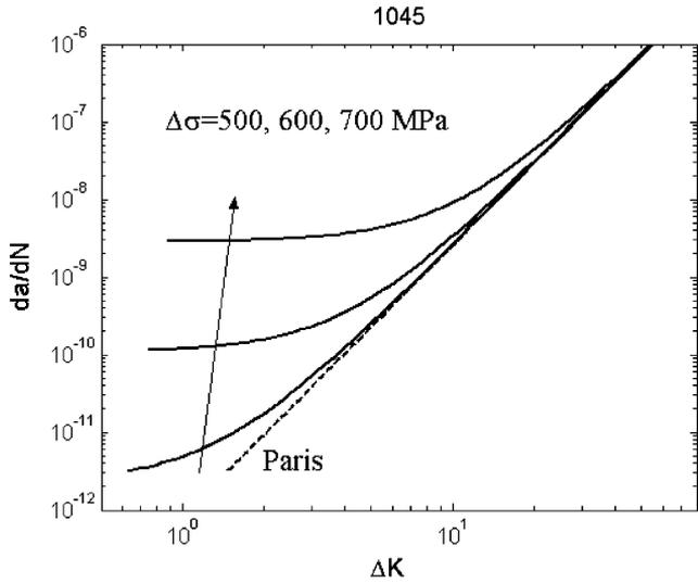
Fig. 5. Crack propagation laws from Eq. (25) with fixed  $\Delta\sigma$  (in MPa in the legend). Notice that with fixed  $\Delta\sigma$  we obtain substantially larger propagation rates.  $\Delta K$  is in  $\text{MPa m}^{1/2}$  and  $da/dN$  is in  $\text{m/cycle}$ .
