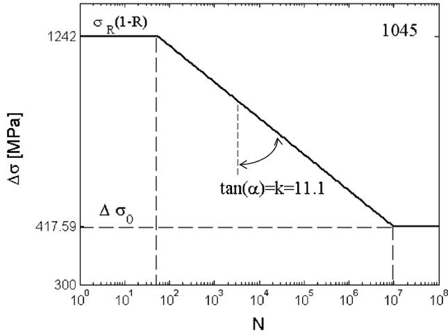
Fig. 1. Schematic Wöhler law (1) for 1045 steel (see example paragraph for the data). Here,  $R = -1$ .
