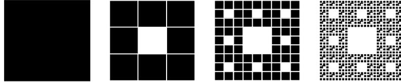
Figure 2. The Sierpinski carpet ( $D=1.89$ ) at different levels of observation; it corresponds to the cross section of a deterministic hierarchical bar in which the white zones represent the soft matrix, and the black ones are the hard inclusions.
