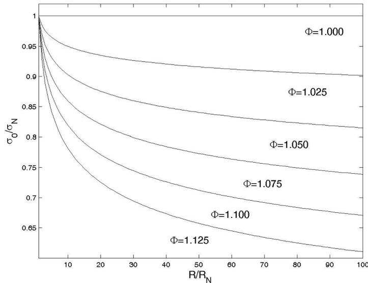
Figure 3. Scaling law of the nominal strength  $\sigma_0$  for different values of  $\Phi$  ( $n = 9$ ,  $n_h = 8$ ). If  $\Phi = 9/8 = 1.125$  the classical Sierpinski carpet is recovered and  $D^* = 2 - (\log 8 / \log 3)$  (Eq. 15).
