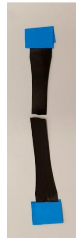
Tensile test on macro samples of graphene composites
